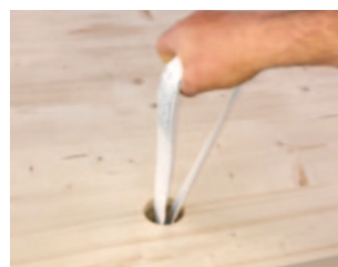
2. Lifting situation with built-in system VLS S1
