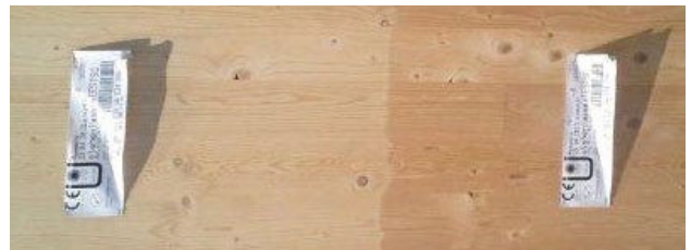
Figure 12. Discolouration due to direct sunlight (UV)
