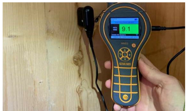
Figure 34. Wood moisture measurement
