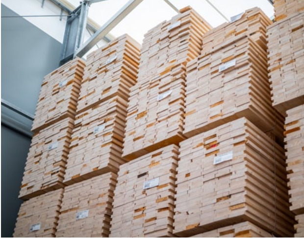
PEFC/06-34-110 - certified lamellae undergo machine strength grading and are sorted according to surface quality
