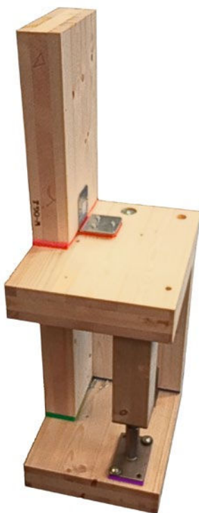
Mockup, sound insulation strips
