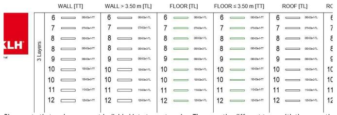
Please note that each component is divided into two categories. These are the different types with the respective cover lamella orientation. By selecting the cover lamella, the orientation of the panel length and width is controlled. In addition, TT and TL types, with the same total thickness, can differ in their lamella thickness.
