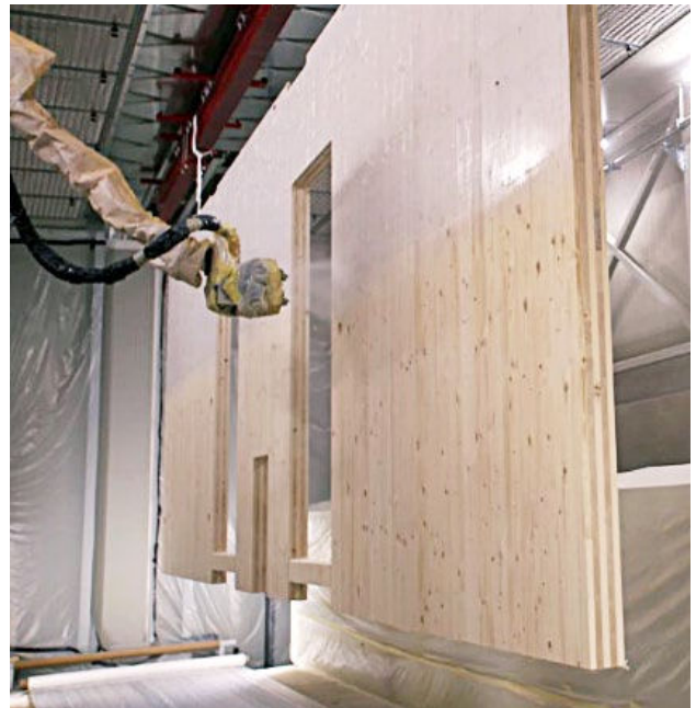
Application of white glazed surface
