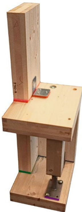
Mockup, sound insulation strips
